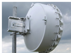
(2+0) system outdoor units directly mounted on the OMT+antenna system
